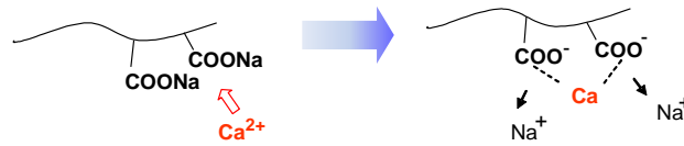
Fig. 7. Hypothesis for mechanism of SFC-Na for trapping calcium (Ca) ion.
