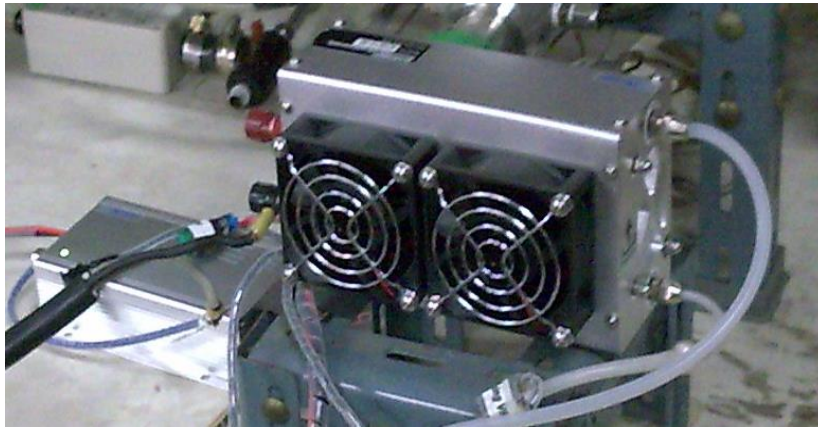
Fig. 3. 200W PEM fuel cell stack.
