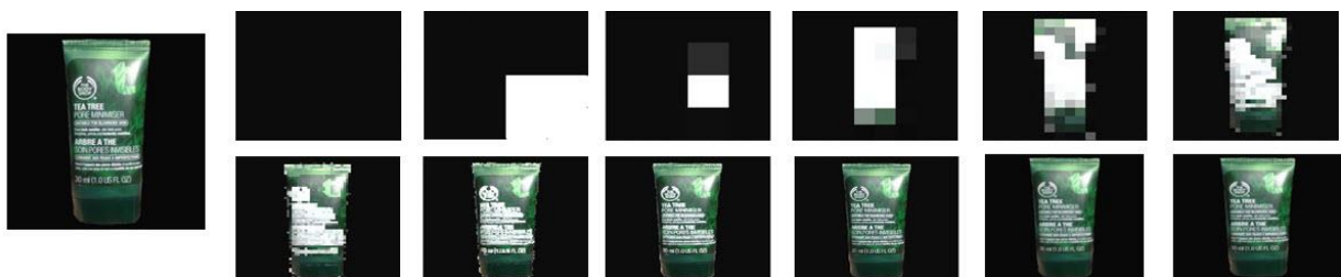
Fig. 10. On the left side is 4096 \times 4096 (2^{12} \times 2^{12}) pixels of input cosmetic Image. On the right side are images from different hierarchy of image pyramid.
