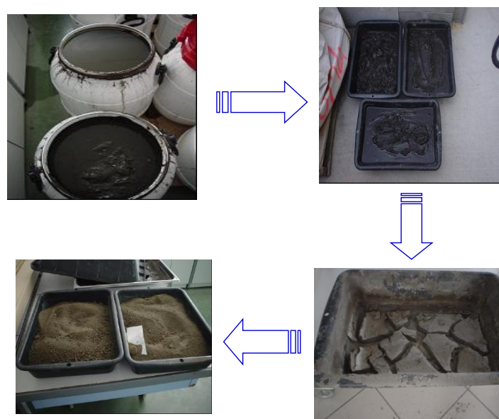
Fig. 3. Sediments preparation steps before their geotechnical characterization.
