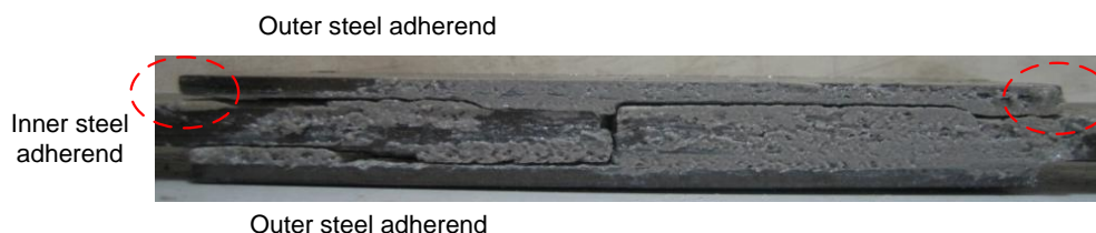
Fig. 7. Debonding failure of specimens.
