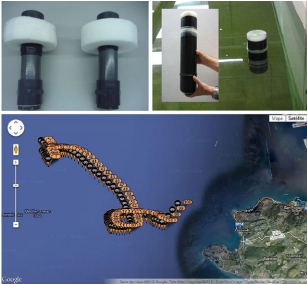
Fig. 16. – Top: first prototype of the PK1 drifter (left) and current design (right). Bottom: trajectory of the first PK1 prototype in deployments in the Gulf of Trieste.
