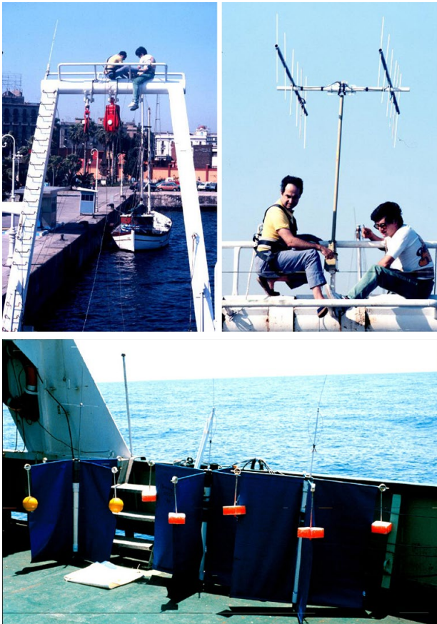
Fig. 1. – Left: Mario Vieira (Marine Sciences Research Centre, State University of New York) and Arturo Castellón (ICM, CSIC) installing the VHF antenna on top of the A-frame crane of R/V García del Cid . Right: a closer look at the VHF antenna for tracking drifters. Bottom: CODE-type drifters used during the FE87 cruise equipped with the characteristic long, thin cross-shaped VHF antenna.
