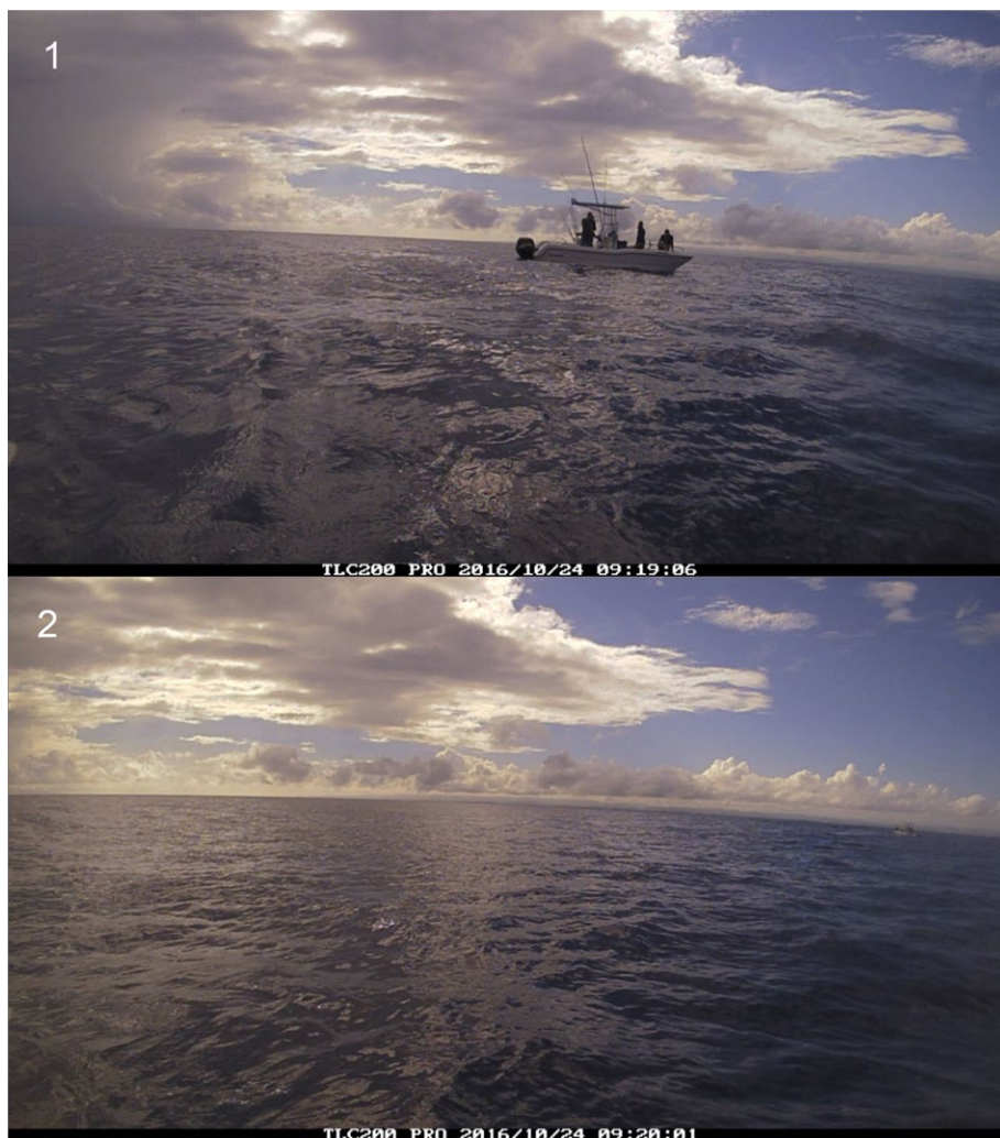
Fig. S1. – A camera was redeployed to conduct a range test to determine approximately how far a vessel in an image was from the FAD. Image (1) is a vessel that is 70 metres from the FAD; Image (2) is the same vessel 132 m from the FAD. These photos were used to determine the proximity of vessels to the FADs.
