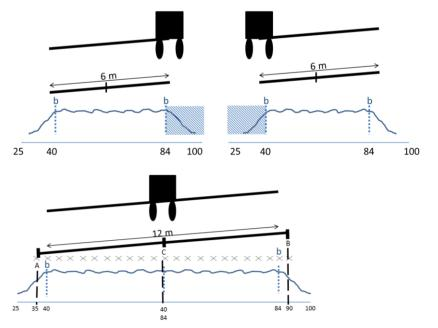
Figure 17 : Simulation of the distribution for a 12 m boom by combination of two half-boom of 6 m. The unwanted edge effects of the center of the boom are removed beyond the tube 84 and before the tube 40. "b" = boundary of the edge effect. Hatched = edge effect deleted from the data. Cross = location of a nozzle
