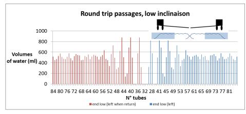
Figure 20 : sprays at the boom ends during two round trip passages: chart shows the decomposition of the liquid sprayed by each of the two passages. Half booms are inclined 5 ° downwards. Working height = 60 cm
