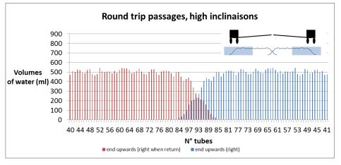
Figure 21 : sprays at the boom ends during two round trip passages: chart shows the decomposition of the liquid sprayed by each of the two passages. Half booms are inclined 5 ° upwards. Working height = 60 cm
