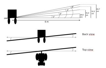
Figure 15 : boom positions into two planes tilts
