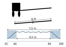
Figure 16 : spray pattern in the 75 collecting tubes. Hatched = edge effect. Numbers under repartition = collecting tube numbers
