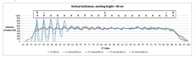
Figure 18 : spray pattern for a ramp inclined vertically. The simulation is carried out from 2 half-ramps of 6 m which meet at point "C" as on Figure 3. "A" = nozzle at the low end. "B" = nozzle at the high end. "b" blue = limits of edge effects. Cross = nozzle location. Working height = 60 cm fixed at point "C"
