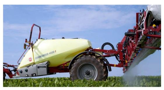
Example of an advanced boom sprayer: HARDI COMMNDER i TWIN FORCE - with ISOBUS Terminal, AutoSectionControl, AutoWash, AutoHeight boom management system and remote data management
