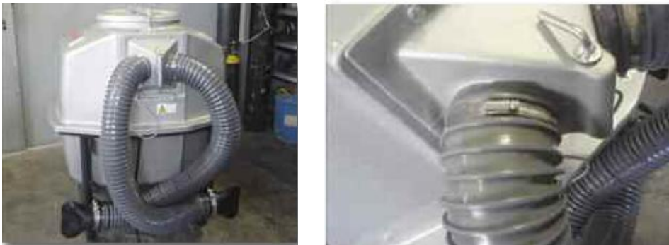
Fig. 16 – Check of the tank leakages using an anemometer
