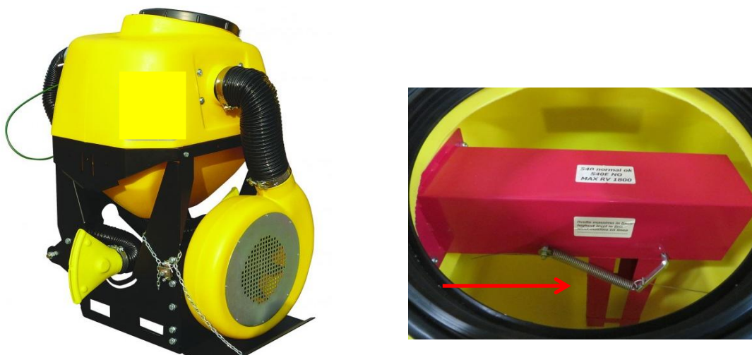
Fig. 12 – Example of agitation system generated by the internal air flow (Photo DiSAFA)
