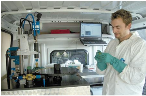
Fig 10: nozzle flowrate & nozzle homogeneity measurement (source GIPPulves)
