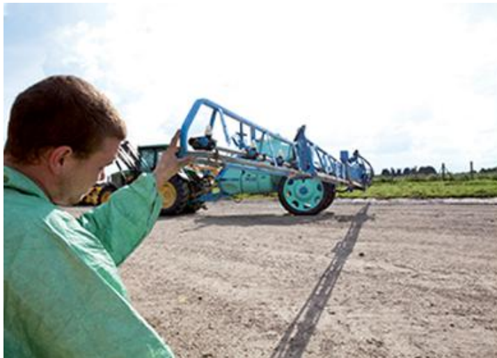
Figure 6: Boom suspension and horizontal tests. Source GIPPulves Along with the boom inspection, the protection of the last nozzle (fig 7) is a mandatory inspection item.
