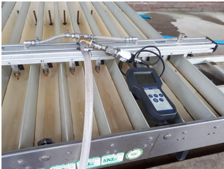
On-site inspection of a mobile patternator
