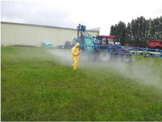
Figure 8: Boom section test, pressure homogeneity test, pressure drop test. Source GIPPulves
