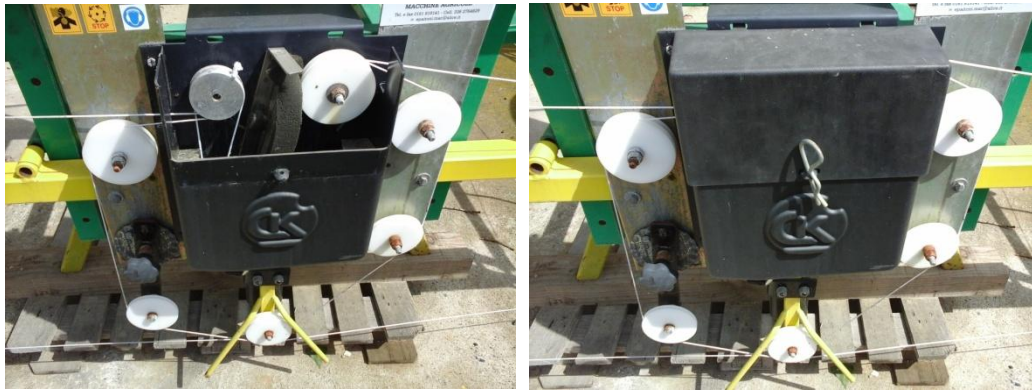
Fig. 5 – Particular of tank for herbicide open and closed whit pulley system (Photo: G. Oggero)
