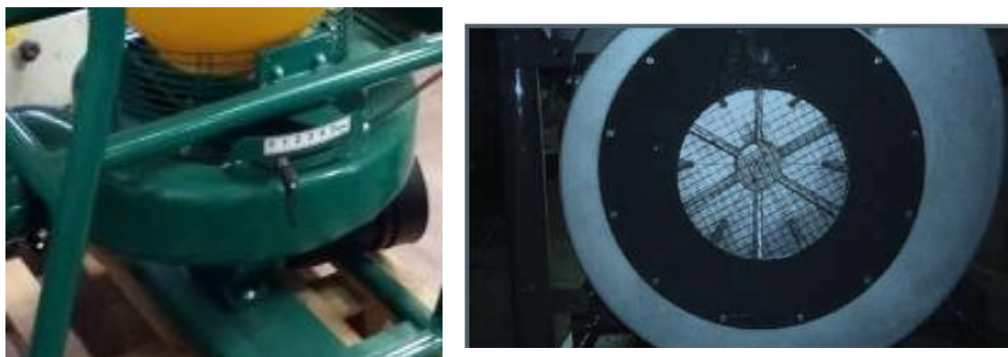
Fig. 5 - Example of the blower and its guarding (Photo: DiSAFA; Spanish manual for the inspection of the sprayers in use)
