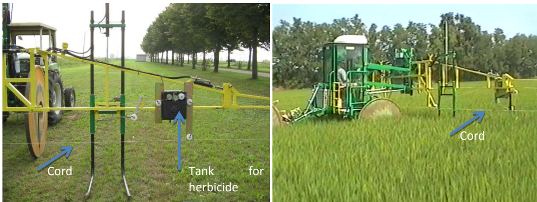
Fig. 3 - Example of weed wiper (distribution of herbicide not diluted using a cord – Type “B” – Photo: MAR snc).
