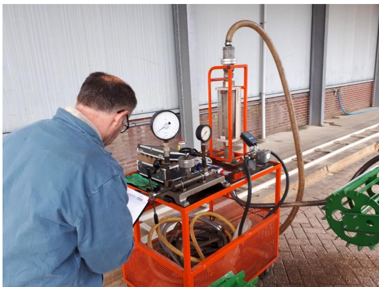
Testing the pump capacity with a certified flow meter
