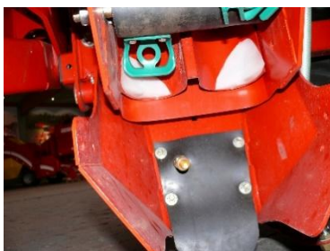
Pic. 9: Mobile spraying on seeds: Potatoe planter with nozzle between hopper and soil
