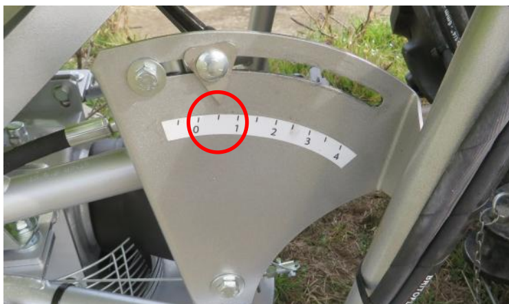
Fig. 14 – Example of device for adjusting the dust rate provided with a zero position that enables to switch off the machine without spreading any dust from the spouts (Photo: DiSAFA)
