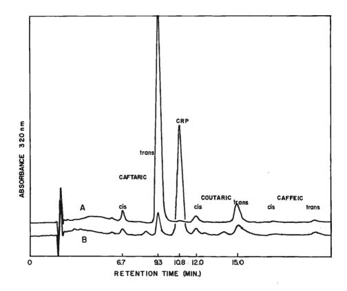
HPLC chromatograms of: A — fully protected fresh Chenin blanc juice, B — the same juice unprotected from air oxidation during crushing.
