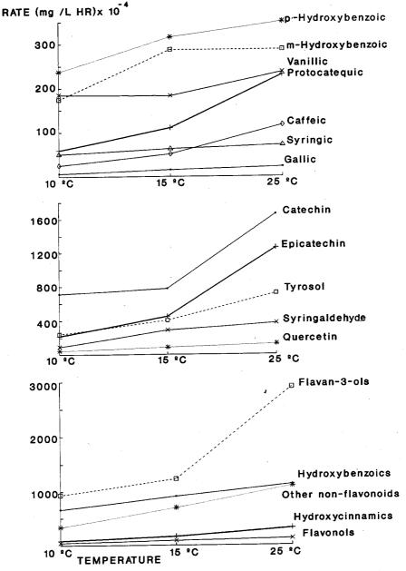
Fig. 1: Changes in the extraction rates of phenolic compounds and fractions as a function of temperature.
