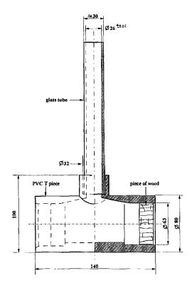
Figure: Experimental half-litre model, developed to allow the extraction of oak wood constituents under conditions similar to those found in full size wine casks (after FEUILLAT *et al.* 1994).
