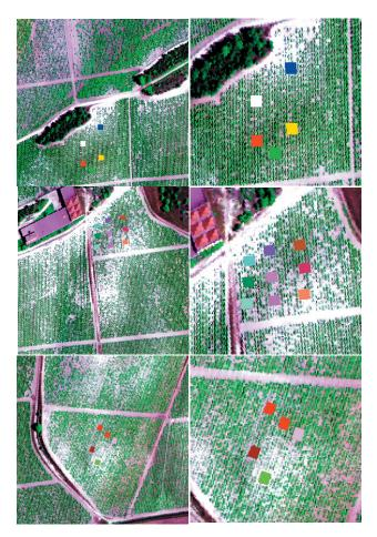
Fig. 1: Airborne hyperspectral CASI images acquired over three of the sites used in this study. The images were collected at 1 m spatial resolution, showing the 10x10 m study blocks used for field sampling collection.
