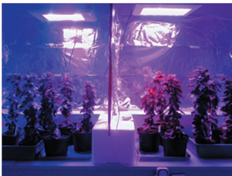
Fig. 1: Experimental set up. Left hand side operating FloraLED® panel, right hand side Blue_Red LED panel.
