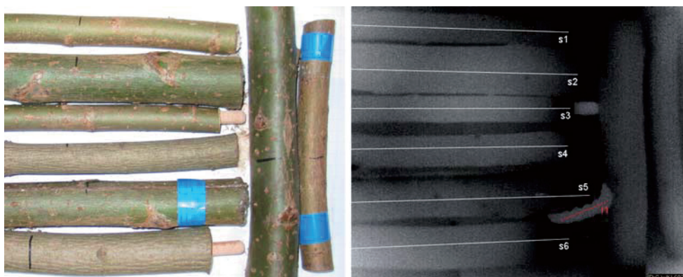
Fig. 4. Thermal test setup of long-term measurement 2. Solid wood samples ( Acer platanoides , Salix caprea ) with axial boreholes in center and inserted Cossus cossus larvae in each sample. Left: Color image with marked positions at the end of boreholes. Right: Thermal image with measurement setup of thermal determination lines (s1 to s6). Test object l1 shows one of two "free" larvae.
