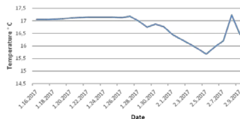
Fig. 4 Average temperature registered during the test in the treatment chamber
