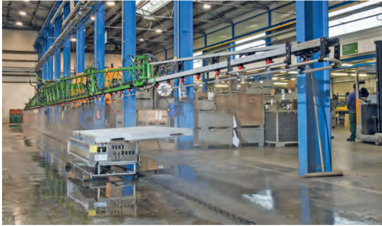
Inspection of cross distribution on test bench according EN ISO 16122
