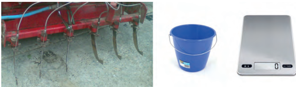
Fig. 4. Soil-disinfection machine injectors, pattern measurement.
