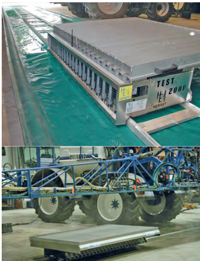
Fig. 5. Examples of electronic horizontal test benches (e.g. “scanner” type).
