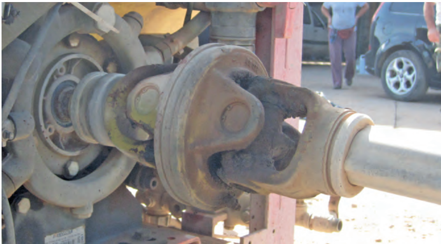
Fig. 2. Absence of PTO shields.
