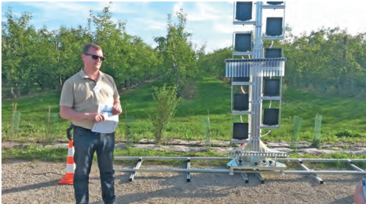
Fig. 6. Demonstration of vertical patternator AAMS-Salvarani.
