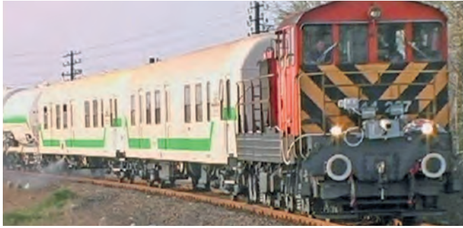
Fig. 1. Spray train spraying the side of the railroad track. The weed detection unit is in front of the locomotive (between the headlamps) (Phot. G&G).
