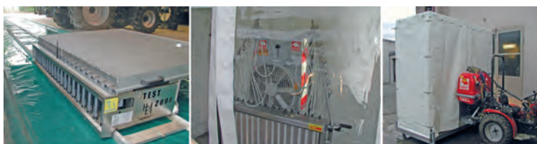
Fig. 5. Examples of systems for collection and disposal of liquid sprayed and for ensuring that there are no leaks of polluting residues generated by the sprayer.
