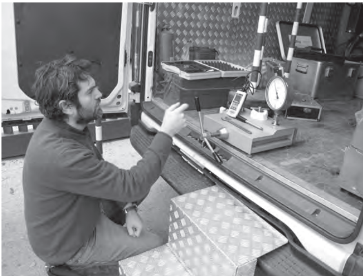
Fig. 1. The function test of a pressure gauge.
