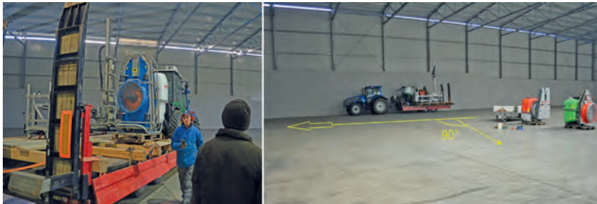
Fig. 4. Test configuration for the air flow measurement with moving tractor.
