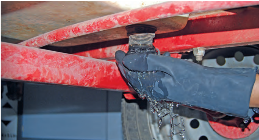
Fig. 4. Impossibility of emptying the tank without losses.
