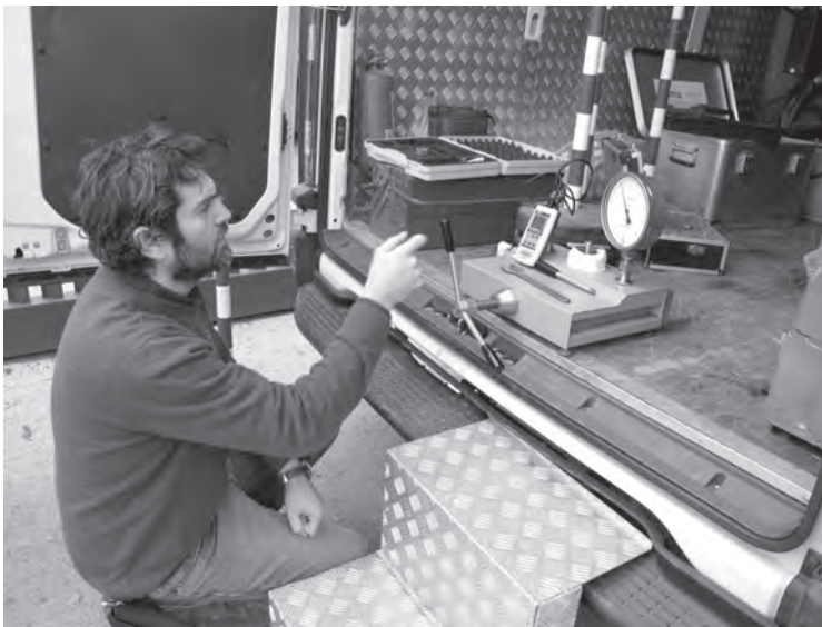
Fig. 1. The function test of a pressure gauge.
