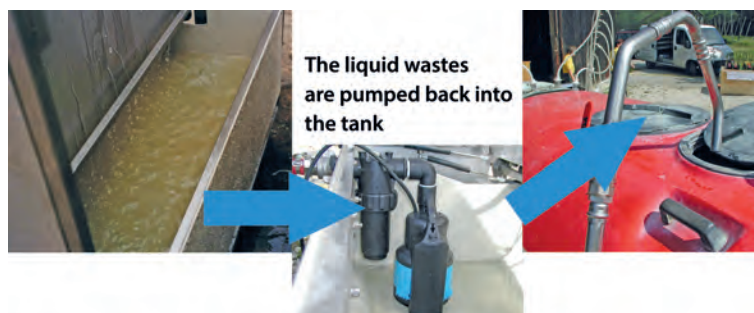
Fig. 6. Example of system for collection and properly disposal of all wastes produced during sprayer inspection/ calibration.
