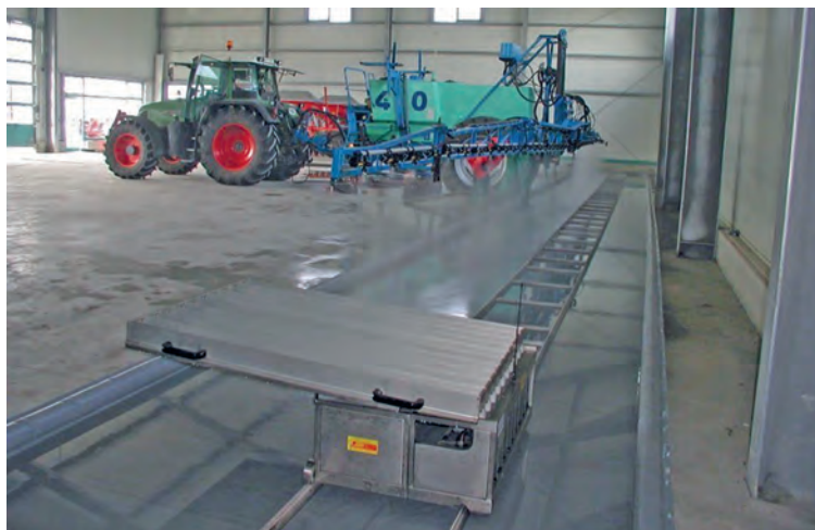
Fig. 4. Place where the inspection/calibration is carried out shall be large enough to accommodate a proper verification of distribution uniformity of the boom throughout its full length.
