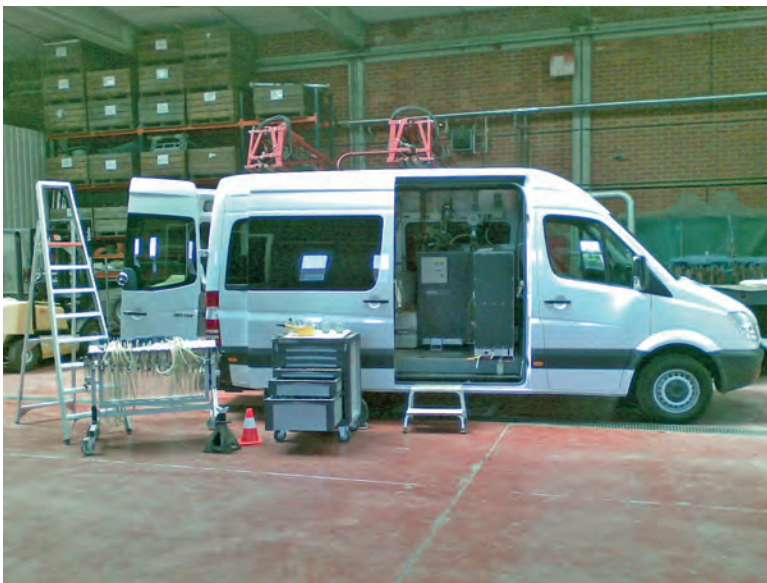
Fig. 1. Inspection van with test equipment.
