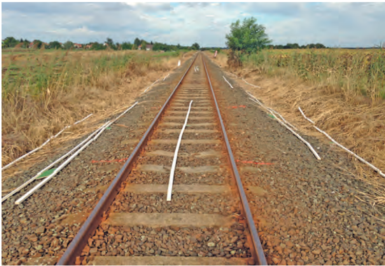
Fig. 5. Measurement of the longitudinal distribution of the spray train with filter paper. (Phot. Wegener).
