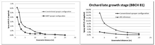
Figure 2. A) Comparison of average spray drift curves obtained in Italian orchards using conventional sprayer configurations and sprayer configurations equipped with SDRT. B) Comparison of the average spray drift curve assessed in the Italian orchards at late growth stage (BBCH 81) with the curve of reference JKI basic drift values.
