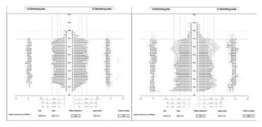
Figure 2: Almost perfect vertical air distribution patterns from orchard sprayers adjusted to a working height of 3.5 m
