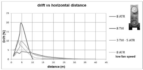
Figure 2. Drift deposition as a percentage of the used water volume in the orchard after application with the cross flow sprayer. Different nozzle types and fan speed were performed.
