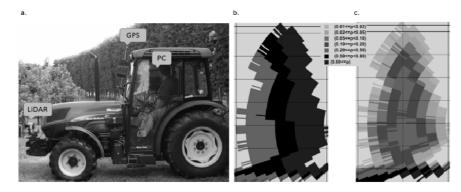
Figure 1. (a) The off-the-shelf systems of a tractor mounted LiDAR Crop Scanner, (b) cumulative probability of the LiDAR beam transmission, (c) local differential probability of the LiDAR beam interception.
