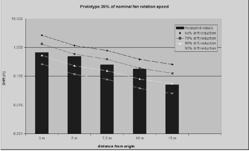
Figure 6: drift behavior Geisenheim prototype
