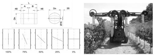
Figure 1. Technical characteristics of the adjustable valve (left) and Iris 1500 L sprayer (llemo Hardi S.A.U.) modified for the trials (right).
