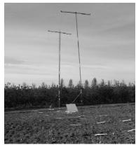
Fig. 2. Horizontal and vertical collectors distribution (ISO 22866), and the mirror.
