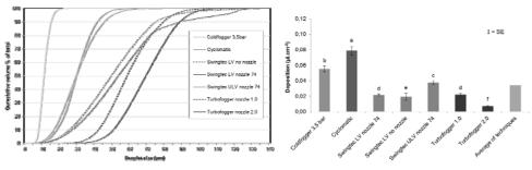
Figure 1. Cumulative volumetric droplet size distribution of the four foggers and different settings used. Measured at 0.50 m from the nozzle outlet.
