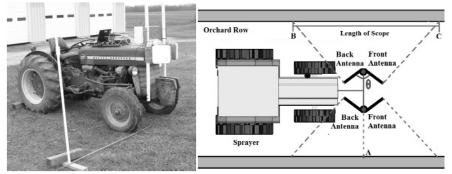
Figure 1. Test tractor
