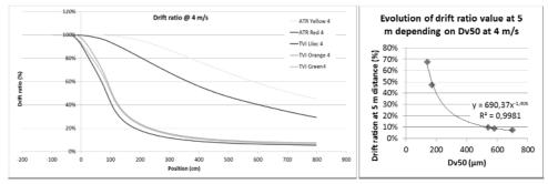
Drift ratio curves (Fig 2a.) are given as an example among the different wind speeds and nozzle orientation tested. A clear discrimination is observed between nozzle types (ATR vs TVI).
