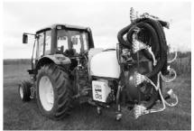
Figure 1. Newly developed automated variable-rate, air-assisted precision sprayer
