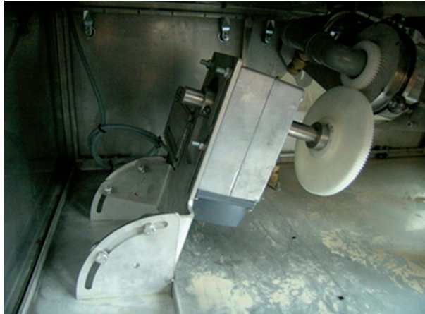
Fig. 3 Details of motor suspension.
