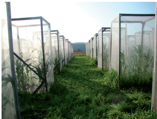
Fig. 1 Isolation cages sized 1.4 m x 1.4 m x 2.5 m (photo: Johann Robier).
