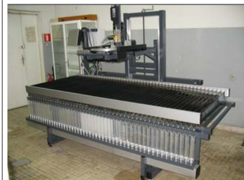
Fig. 3. Device to complex measurements of agricultural nozzles
