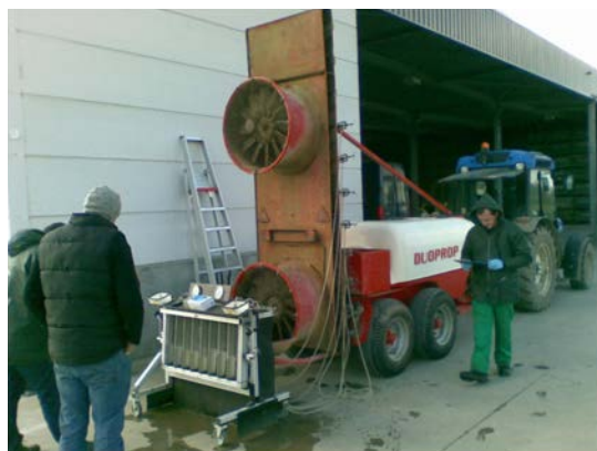
Fig. 1. Measuring nozzle flow rate and spray pressures.
