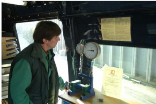
Fig. 5. Testing the sprayer manometer.
