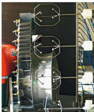
Fig. 1. Device for air flow measurements.
