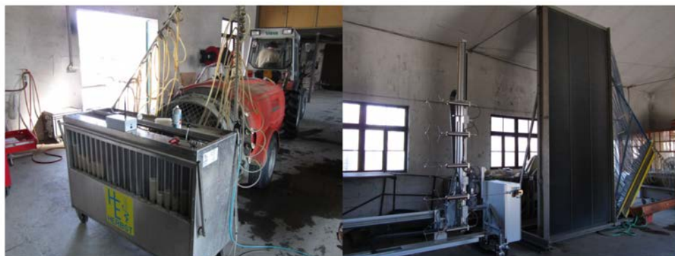
Fig 1. Test bench for the measurement of the flow rate of each nozzle (left) and of the liquid distribution (right).
