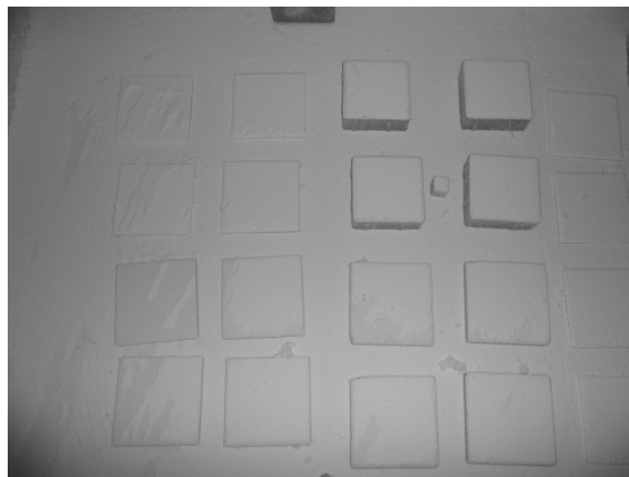
Figure 2 Different surface materials after empty room treatment with diatomaceous earth SilicoSec in field trial, before exposing and caging of insects.
