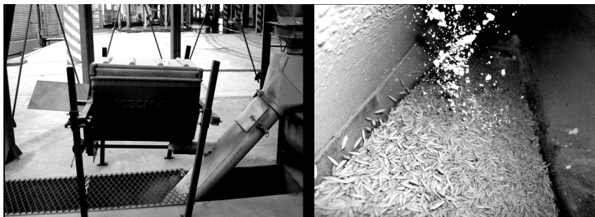
Figure 3 Application of diatomaceous earth + deltamethrin on the rice transported to the silos. Silos floor and internal walls were treated as the treated rice mass dropped from 25 m high.
