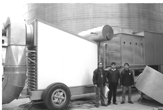
Figure 4 Artificial chilling equipment used to insufflate chilled air through the aeration system of the silos.
