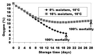
Figure 5 Average percentage oxygen for three replications at 8 and 16% maize moisture and 10°C.
