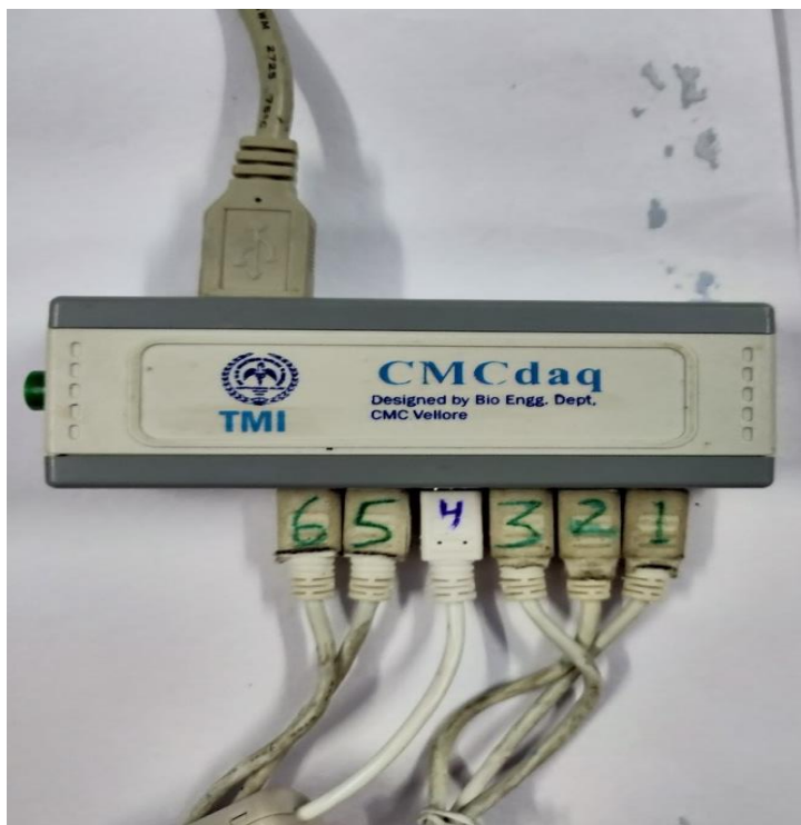
Figure 13. The indigenous CMC data acquisition system with input from all six channels and output routed to a laptop
