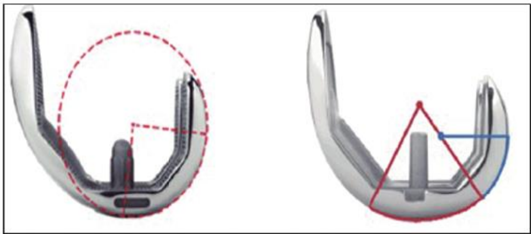
Schematic description of a single radius prostheses (left) and a multi radius prosthesis (right) with their rotation axis [14]. (License number: 2734170007640).
