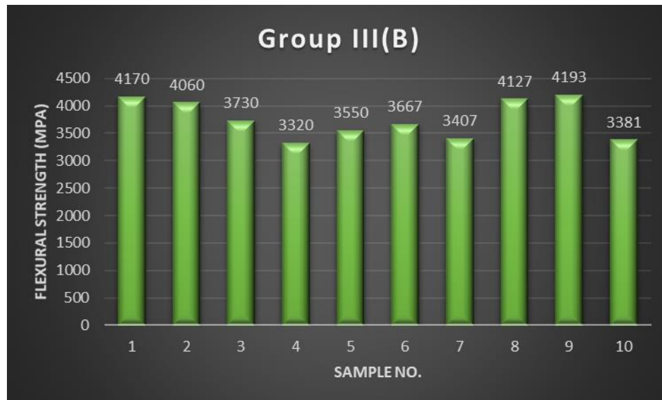
Graph: 6 Basic values of flexural strength of PEEK after 14 days of aging and 1000 cycles (Group III (B)).
