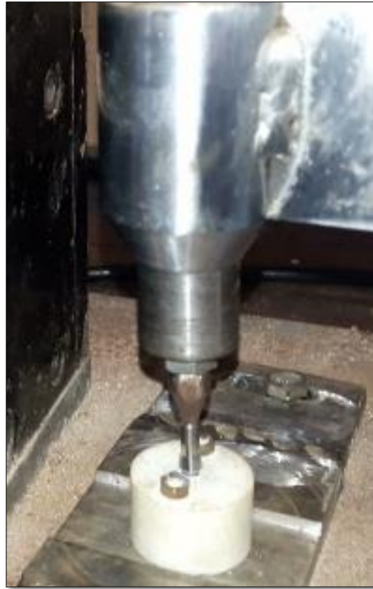
Fig .24: Cyclic loading of Titanium abutment sample
