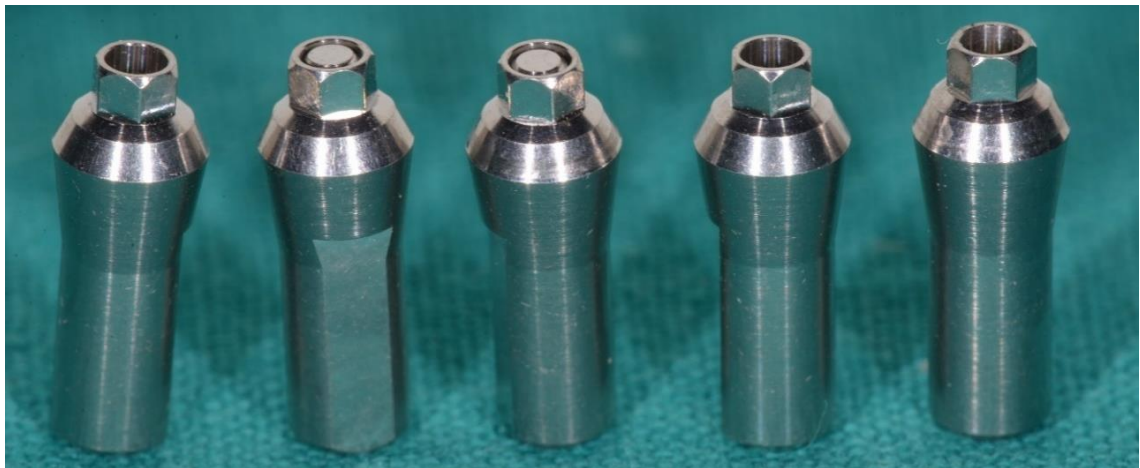
Fig:31:Observation of post cyclic loaded Titanium abutment
