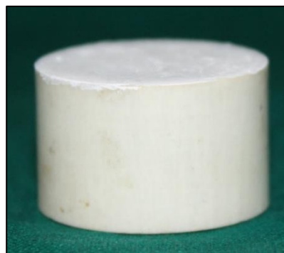
Fig.2: Fibre reinforced epoxy resin block of 16×25 mm dimension
