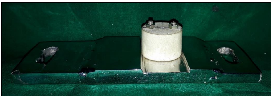
Fig .9:Customized jig attached to resin block
