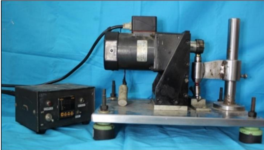
Fig. 22 :Customized Cyclic loading machine with Timer
