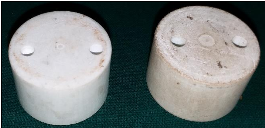
Fig.7:3 mm Parallel holes drilled in the block
