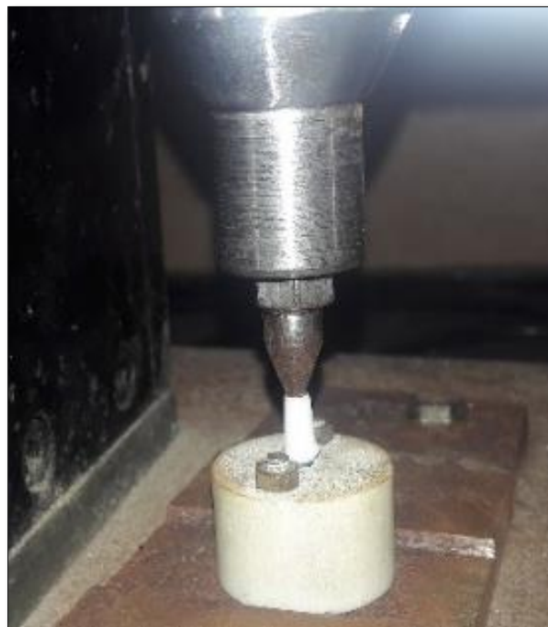
Fig.25: Cyclic loading of Zirconia abutment sample
