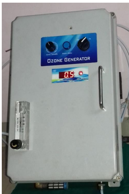
Figure 3. Ozone generator for preparation of ozonated water
