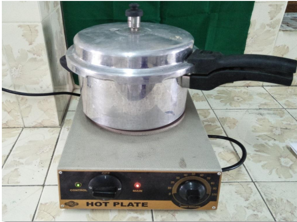
CP 7: Pressure cooker for antigen retrieval
