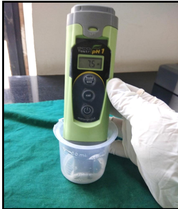
Figure 10: The tip of the pH bulb was immersed in the calibrated cup containing salivary solution
