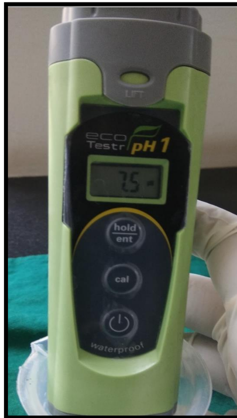
Figure 3 : pH meter used for SFR and salivary pH analysis
