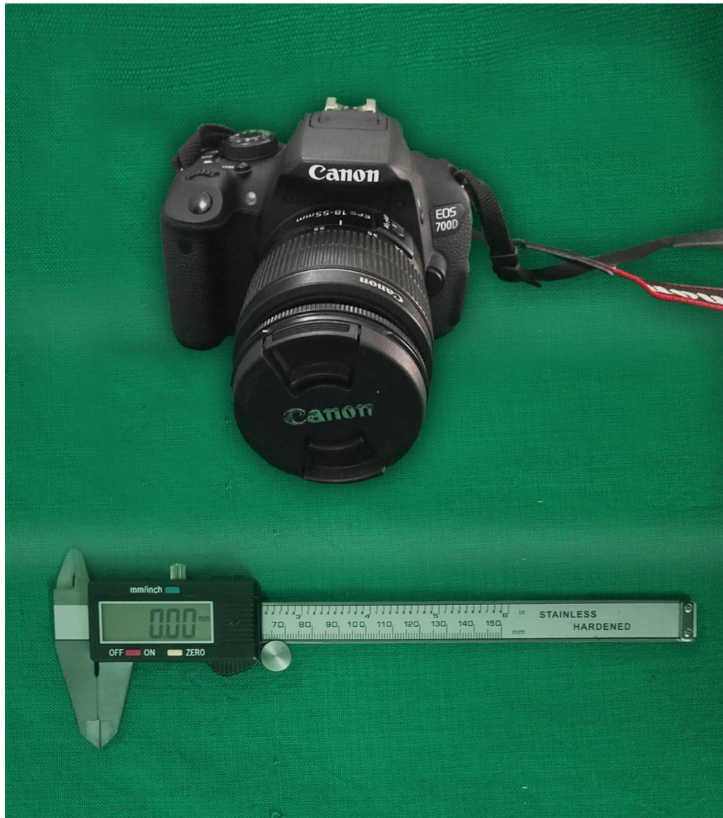
Figure 3: Digital vernier calliper and a Digital SLR Camera used to measure Shimbashi number and to take photograph
