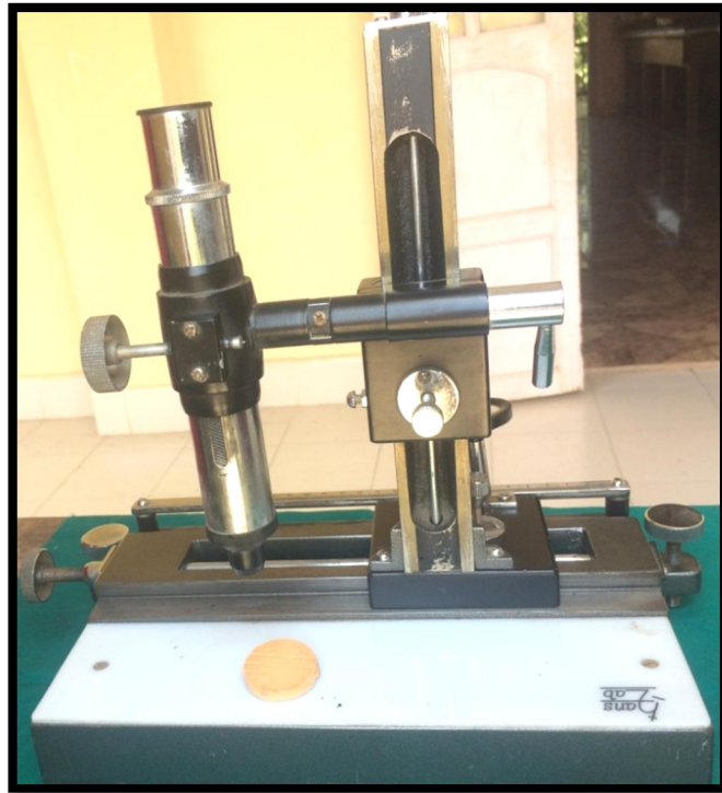
Fig:13 Dimensional stability evaluation through travelling microscope
