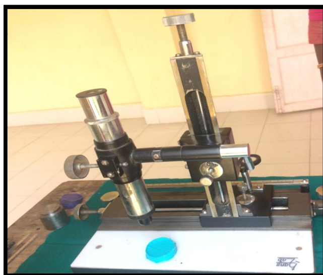
Fig:12 Smooth surface evaluation through travelling microscope
