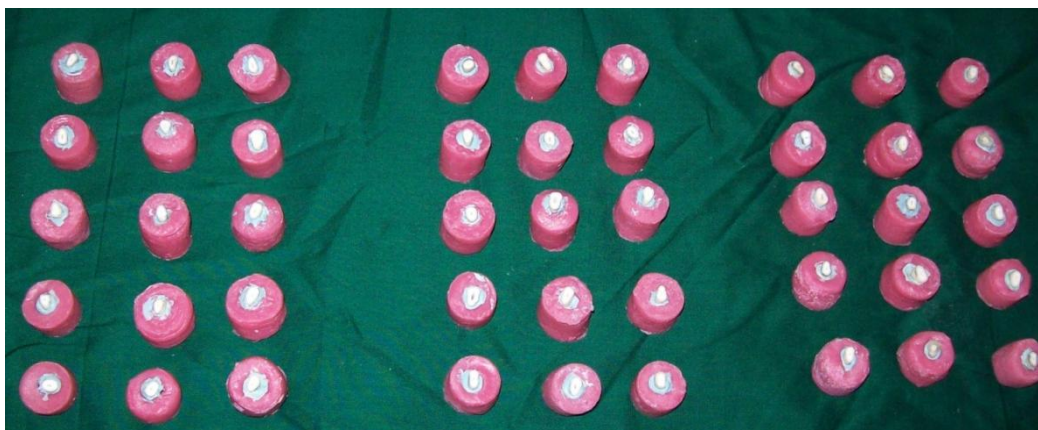
Fig 12: POLY VINYL SILOXANE COATED SPECIMENS WITH IN ACRYLIC RESIN MOULDS
