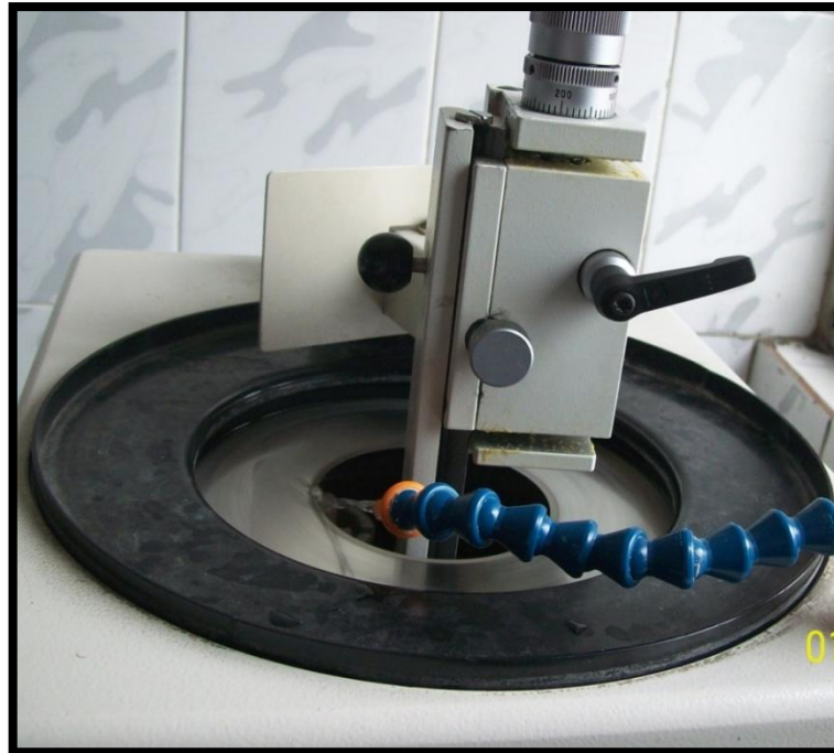
Fig 19: SECTIONING OF SPECIMENS WITH HARD TISSUE MICROTOME
