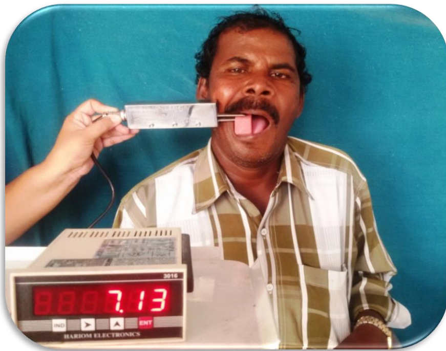
Figure 16: BITE FORCE AT 30 MM VERTICAL DIMENSION
