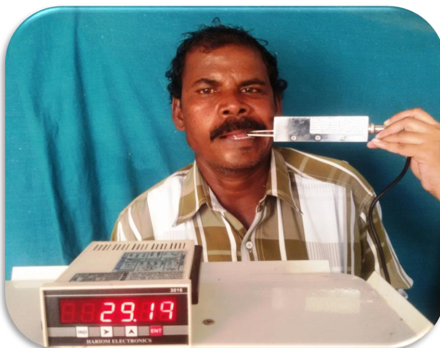
Figure 11: BITE FORCE MEASUREMENT IN LEFT MOLAR
