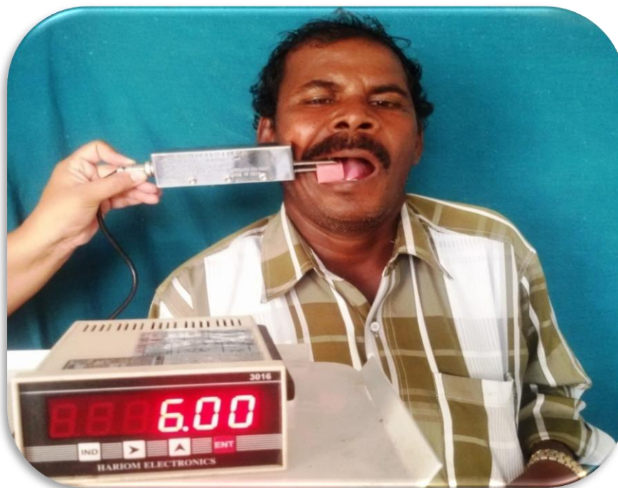
Figure 15: BITE FORCE AT 25 MM VERTICAL DIMENSION
