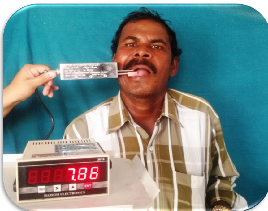
Figure 13: BITE FORCE AT 15 MM VERTICAL DIMENSION
