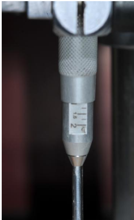
Figure 15- Torque level kept at 1kg.cm during insertion
