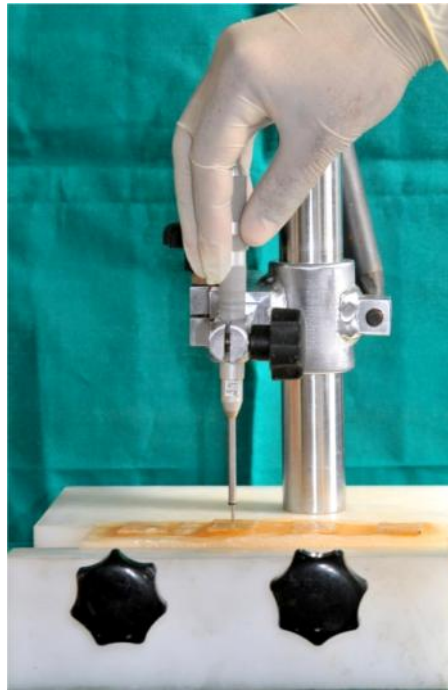
Figure 14- Stand with bone, mini implant and driver
