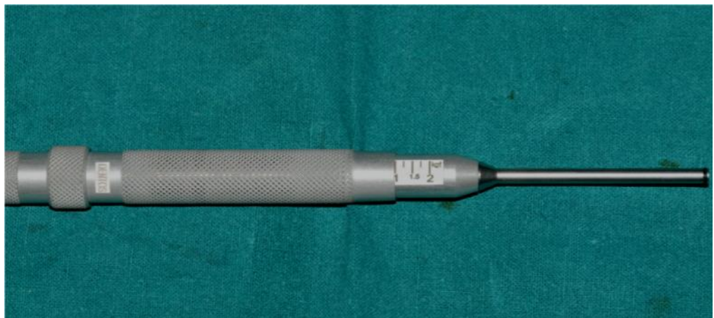
Figure 11- Torque set at 1kg.cm
