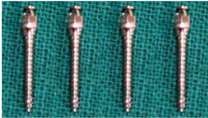
Figure 4-Length 10mm- diameters from left to right-1.3mm, 1.4mm, 1.5mm, 1.6mm
