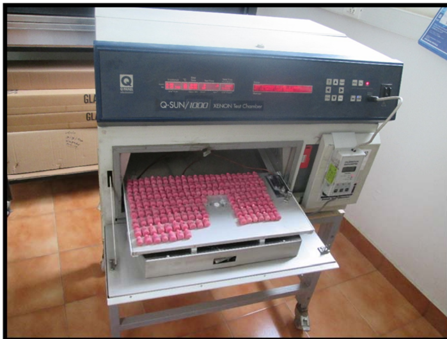
Figure 8: Q-Sun Xe-1B photo ageing apparatus with the tooth samples
