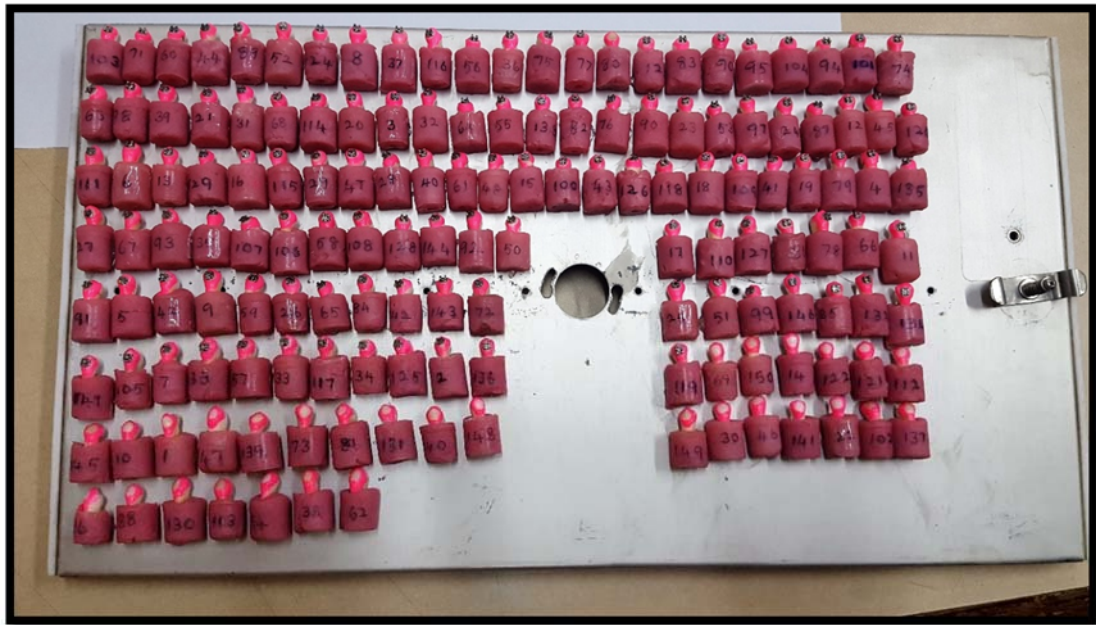
Figure 7: Samples attached with brackets and fixed on to tray for photo ageing
