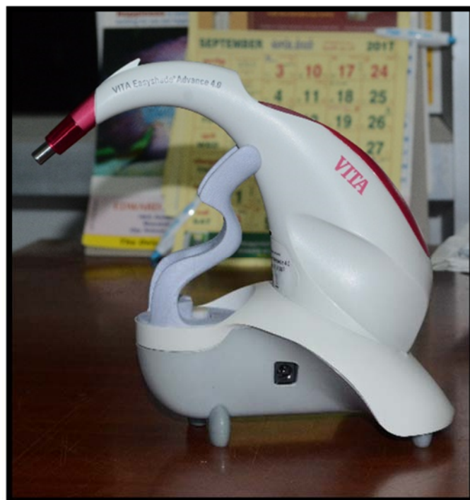
Figure 6: colour evaluation using spectrophotometer (Vita Easy Shade Advance 4.0)
