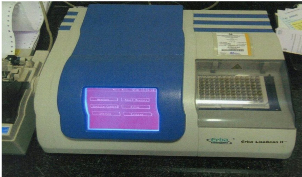
Image 10 : Spectrophotometer (ELISA Reader) with Microtiter plate
