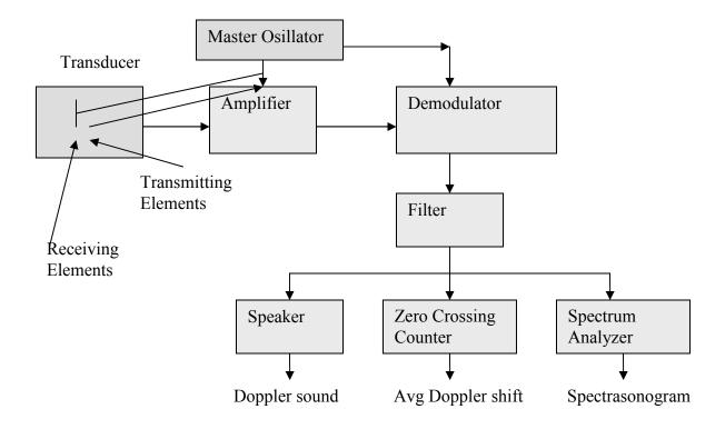
Fig 1: Block diagram of a CW Doppler flow meter
